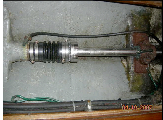
Dripless shaft seal & pillow block bearing
